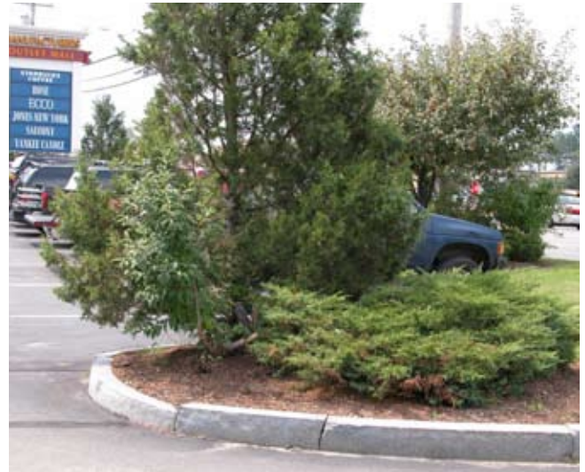
The ultimate height and density of these plantings were not considered in the planting plan, resulting in a potentially dangerous blind spot for someone backing out of this parking space.
