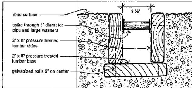
**Open Top Culvert:** Use this structure in a sloped gravel driveway or camp road that does not get plowed in the winter. Place it at a 30 degree angle to the road edge and point the outlet into stable vegetation. Remove leaves and debris annually.
