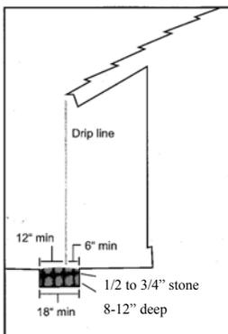
**Dripline Trenches:** Install a rock-filled trench along the roof drip line to collect and infiltrate roof runoff, thereby controlling erosive runoff from the rooftop. The trench will collect roof runoff and store it until it soaks into the soil. These systems will also reduce wear on your house by reducing back splash.
