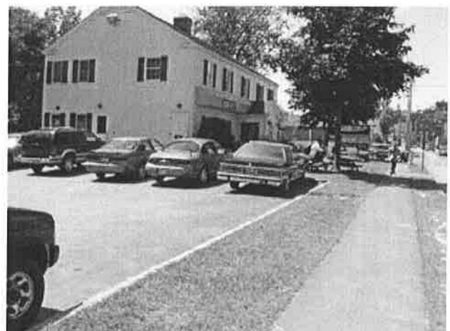
Dead-end parking lots are difficult to exit, especially when the lot is full.
