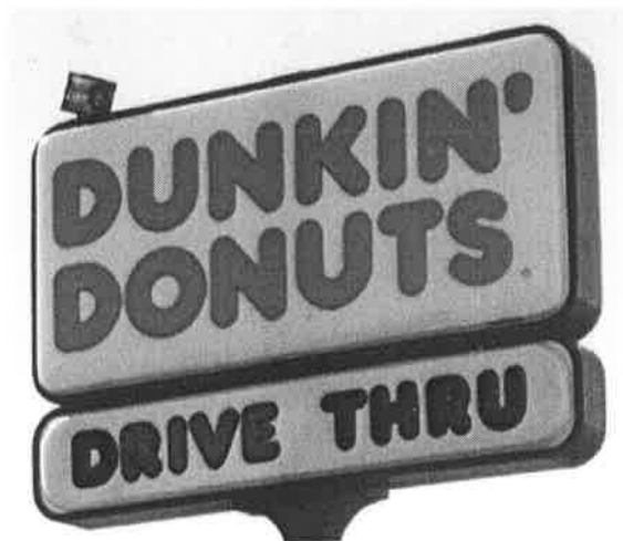
This message of the sign should be translucent, and not the white background as in this example.
