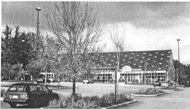
Parking lot islands should be large enough for trees to achieve full maturity and to prevent damage from car doors and snowplows.
