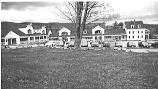
Grade changes and a stone wall were used to screen the parking lot of this new commercial development.
