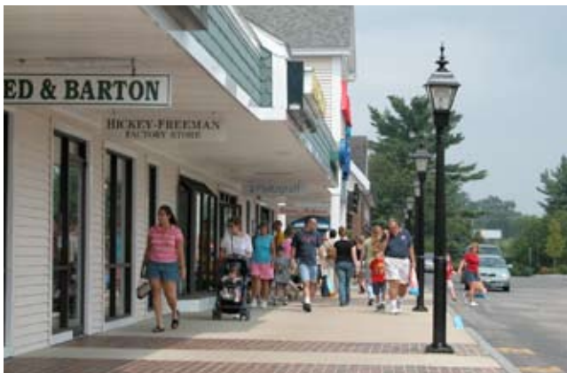
Highly detailed ornamental lighting, mounted on 10' poles, is in scale with the pedestrian environment.
