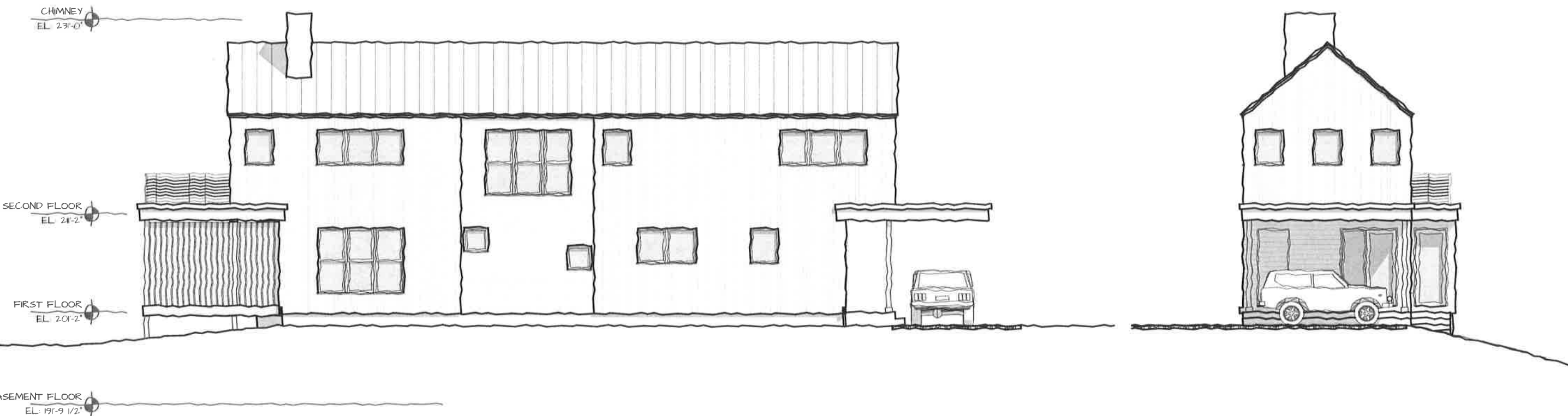
EAST ELEVATION (STREET SIDE) 3/32" = 1'-0"
