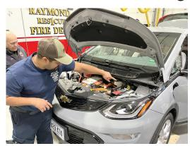
A 40 Minute PPT presentation and review of reference guides from NFPA concluded with a 40-minute review of the town's electric vehicle the Chevy Bolt. The Bolt was raised on blocks so the battery area could be reviewed. Students identified electrical disconnects, which wires were safe to cut for power if needed, and reviewed the safety features like airbag systems, and procedures for responding to incidents involving EV's.
