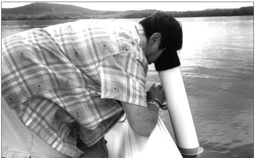
(Measuring) Testing lake clarity with scope and Secchi disk.
