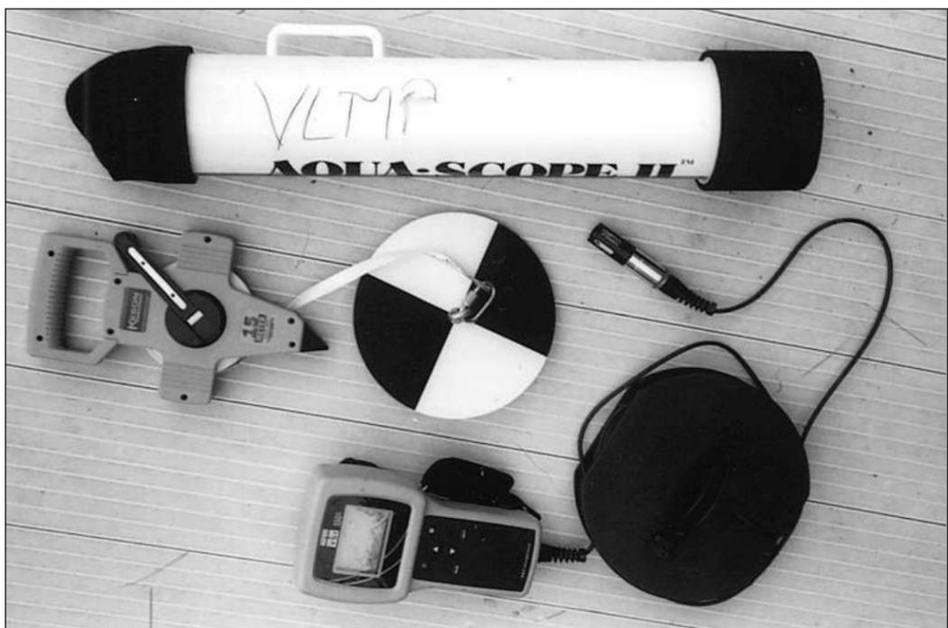
(Tools) Water quality testing tools, clockwise from top: scope, probe and cable, O2 meter, Secchi disk and reel.
