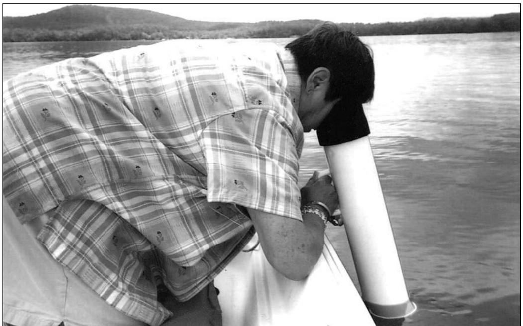
(Measuring) Testing lake clarity with scope and Secchi disk.
